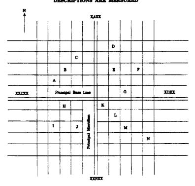
In each state using the rectangular system of surveys there are drawn arbitrary lines perpundicular to each other, one called the 'principal base line' running costs and west and the other called the 'principal meridian running north and south. Townships are measured north and south of the principal base line and ranges are measured east and west of the principal meridian. Each of the squares indicated in the above chart lettered from A to N indicates a township air miles somes.
