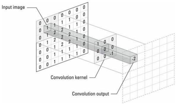
**FIGURE 11-5:** A convolution scanning through an image.
