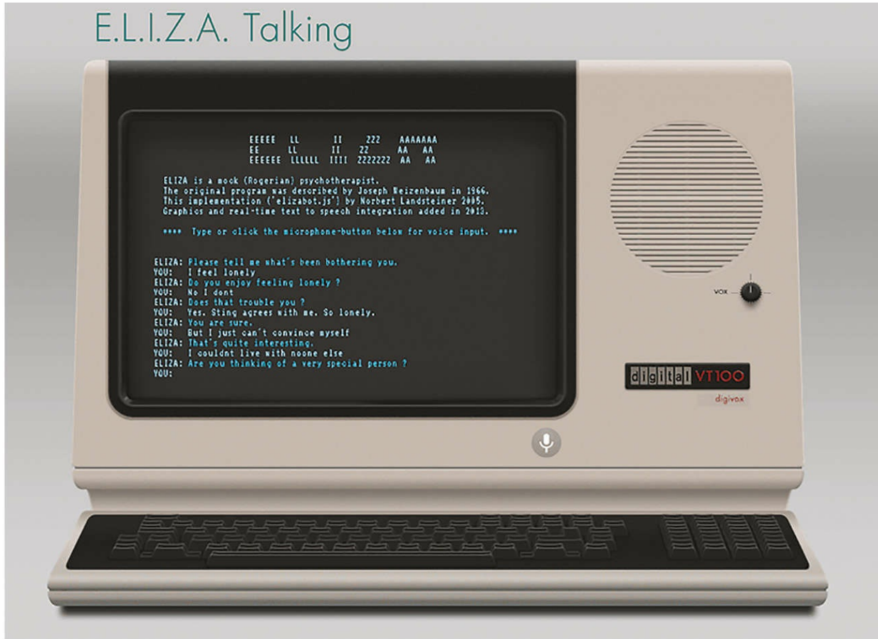
Fig. 14: ELIZA – The First Chatbot. Developed by Joseph Weizenbaum in 1966, ELIZA simulated human-like conversation using pattern-matching techniques, sparking early debates on AI's ability to understand language and emotions.
