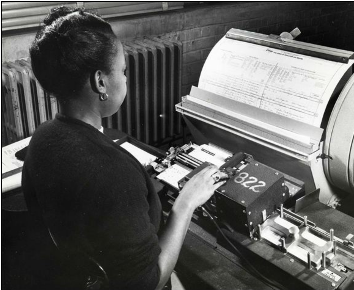
FIGURE 2-4: A tabulating machine and its operator add results from the 1950 census.
